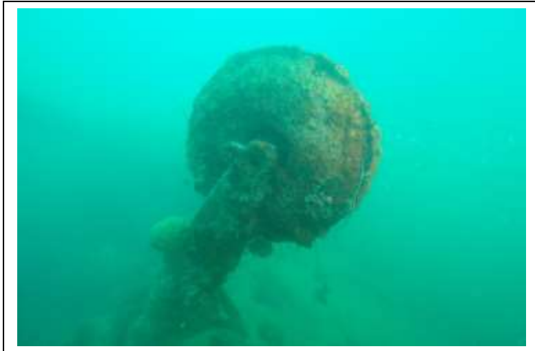
Figure 7. One of the fixed undercarriage wheels of the Val Dive Bomber. Photo Ewan Stevenson.
