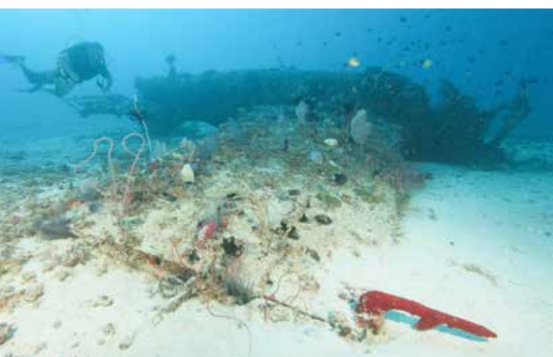
Figure 35 and 36. Left: Matt Wray studies the tail area. The pitot tube (airspeed measurement device) is amazingly prominent. It is completely covered in growth, yet curiously appears to be the correct colour as per the Grumman Engineering Aircraft Corporation Maintenance Instruction for the F4F-4 airplane, Note 18 on p. 228 "Paint Pitot tube, non-specular red, in accordance with E.A.L. process spec. #1647". It is not known for sure, but it appears the marine growth on the pitot tube may have assimilated the red pigment out of the paint. As often found on Wildcat sites in the Solomons, the wing tip cap, Part No. 10864, is missing. Right: This rear view shows the amount of space under the wings. The starboard wing is entirely just off the seafloor. Chrome Molybdenum steel arresting hook is fully retracted into the tail cone, Part No. 11074. [30 August 2018].
