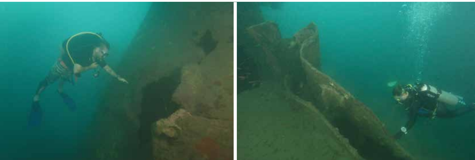
Figure 45 and 46. Left: In the murky depths off Lunga Point, Matt Wray examines the shattered starboard hawse pipe of the upside down bow of the USS Serpens. The Serpens is one of the largest MIA cases in the Solomons with 196 missing. It appears the blast from the explosion vented through the hawse pipe as this is severely cracked in this high-strength area, and peeled it outwards. Right: More evidence of a tremendous blast. This wrinkle in the starboard hull extends vertically from the keel to the bulwark and forms a massive 'buckle' in the hull plating. [1 September 2018].
