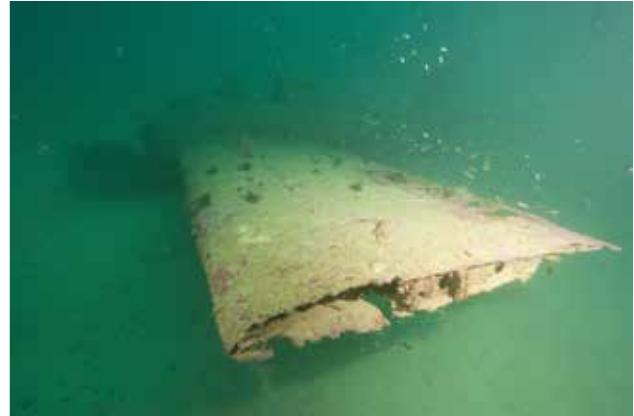
Figure 23 and 24. The port wing tip 27 November 2014 and 28 August 2018, confirming missing pitot tube. The wing tip cap, Part No. 10864, is also missing but was so when originally first dived by Ewan Stevenson on 9 November 2011.
