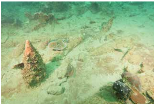
Figure 8 and 9. Left: The different coloured marine growth on the nose of this projectile indicates it's fuzed, and likely a HE Mk. 24 HC round. Right: The photographer's hand holding a sample of smokeless propellant grains.
