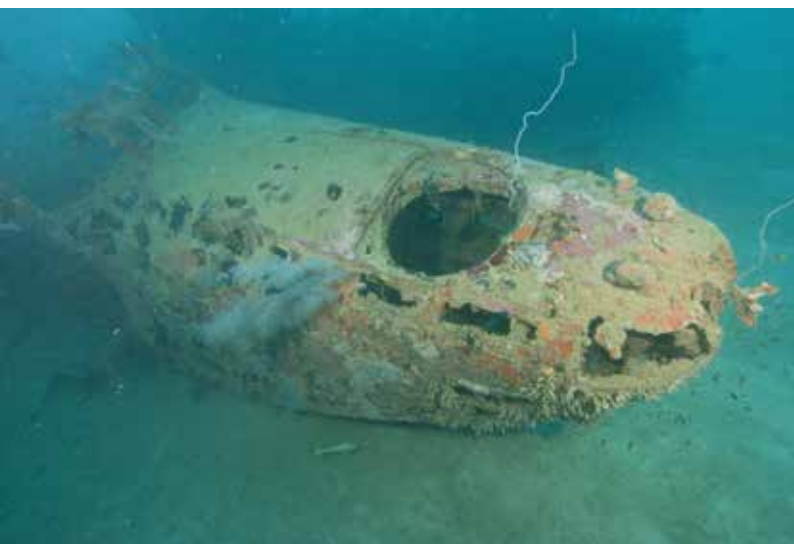
Figure 15 and 16. The nose and Mitsubishi Kensei Engine No. 4 of the MUNITED MAVIS. A hatch cover originally slid over the front gunner's aperture. When Ewan Stevenson first dove the site in January 1999, a full magazine pan for the gunner's 7.7mm Type 92 MG sat on the gunner's seat. "It was an amazing sight. It looked like the gunner had left a few minutes before and absent-minded forgotten it on the seat..." recounted Ewan. On this latest dive, nearly two decades later, the magazine had disappeared. Ewan continued, "It's a shame. I guess it was too tempting for someone to disturb or souvenir, but it reinforces that these sites when first found should be recorded in detail, so these interesting aspects might be preserved so others can share the experience of seeing these poignant aspects..." [27 August 2018].
