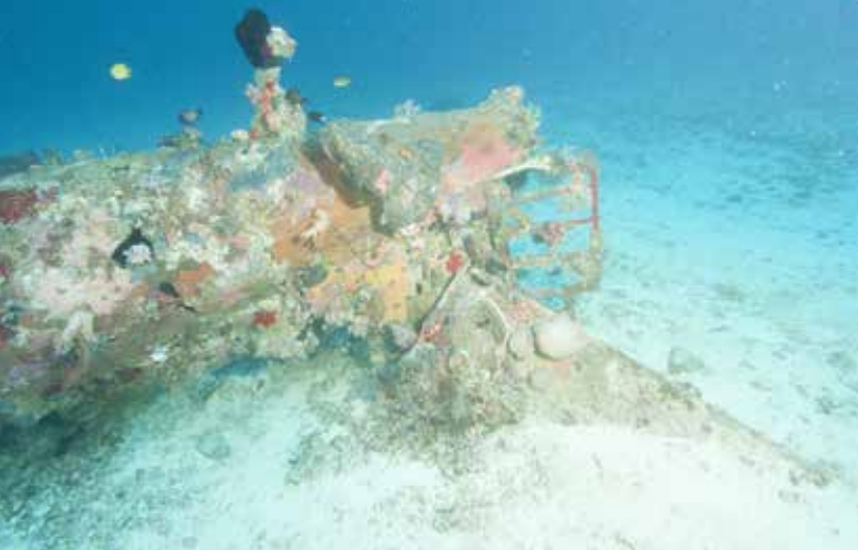
Figure 33 and 34. The collapsed starboard horizontal stabilizer is the most obvious damage on site. The starboard elevator, Part No. 11375, is missing completely, as is the rudder trim tab, Part No. 11392. The B.F. Goodrich 6-ply Heavy Duty 10" pneumatic tyre is missing from the Bendix Tail wheel assembly, Part No. 55612, its place being taken by a Black Feather Star Colobometra perspinosa . The feather star has found the perfect position to filter feed from the ambient current. The right photo shows the underside of the port wing. The oval fairing is for the 10-inch oil cooler, which kept the oil at about 65°C. To the right of the oil cooler air intake is the wing fold line. [30 August 2018].
