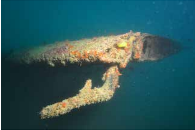
Figure 23 and 24. The port wing tip 27 November 2014 and 28 August 2018, confirming missing pitot tube. The wing tip cap, Part No. 10864, is also missing but was so when originally first dived by Ewan Stevenson on 9 November 2011.
