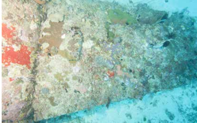
Figure 33 and 34. The collapsed starboard horizontal stabilizer is the most obvious damage on site. The starboard elevator, Part No. 11375, is missing completely, as is the rudder trim tab, Part No. 11392. The B.F. Goodrich 6-ply Heavy Duty 10" pneumatic tyre is missing from the Bendix Tail wheel assembly, Part No. 55612, its place being taken by a Black Feather Star Colobometra perspinosa . The feather star has found the perfect position to filter feed from the ambient current. The right photo shows the underside of the port wing. The oval fairing is for the 10-inch oil cooler, which kept the oil at about 65°C. To the right of the oil cooler air intake is the wing fold line. [30 August 2018].
