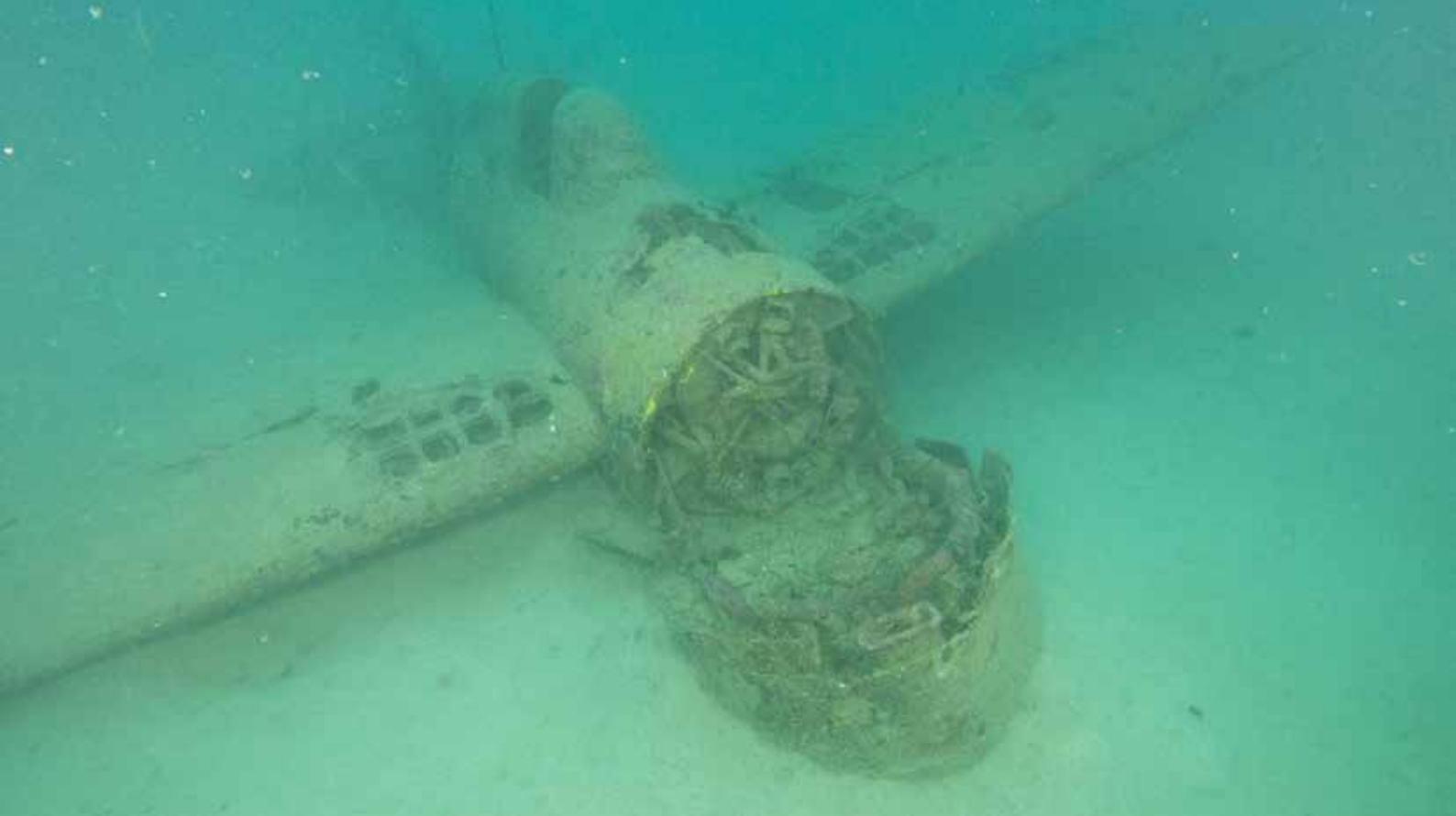
Figure 20. The Gavutu Wildcat. The heat-treated, Chrome Molybdenum steel engine mounts have given way and the Pratt and Whitney Model R-1830-86 radial engine has fallen forward. The combined archaeological evidence indicates this Grumman F4F-4 Wildcat is that of ace-in-a day 1st Lt. James E. Swett's of VMF-221. Part of that evidence is hidden below the sand... Ewan Stevenson predicts the three-bladed Curtiss Electric Model C5315S propeller will not be 'feathered'; and all the hollow steel blades will be perfectly straight... in line with Swett's account. This might explain why no propeller blade is protruding above the sand. Swett related his engine seized due to battle damage on 7 April 1943, "I... managed to get over the bay at Tulagi before the engine froze up. That old propeller blade was sticking straight up right in front of me like the middle finger of the right hand." So, Swett made a dead-stick water landing and there should be a prop blade straight up buried in the front of that engine. [28 August 2018].
