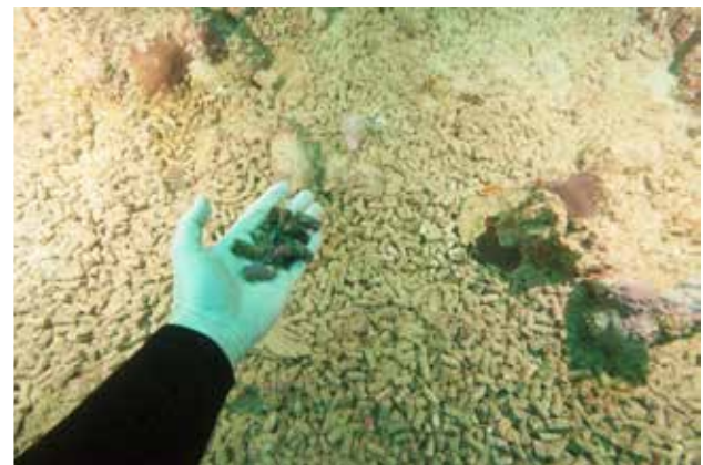
Figure 8 and 9. Left: The different coloured marine growth on the nose of this projectile indicates it's fuzed, and likely a HE Mk. 24 HC round. Right: The photographer's hand holding a sample of smokeless propellant grains.
