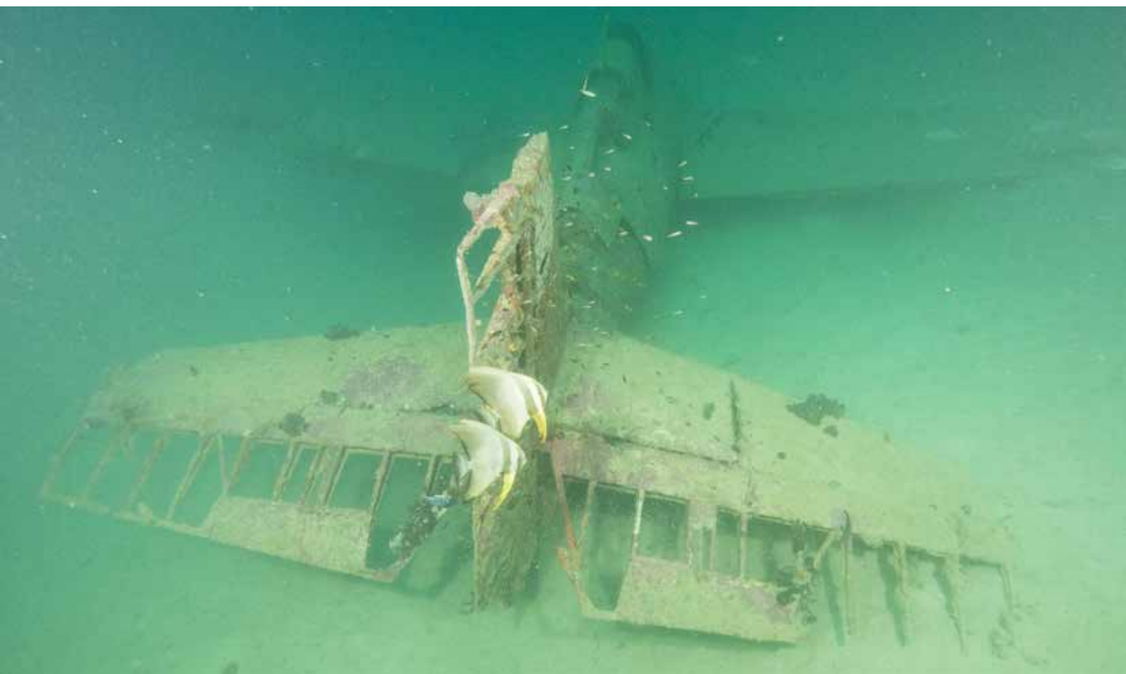
Figure 21. A pair of tall-fin Batfish Platax tiera patrol the tail assembly of The Gavutu Wildcat. The doped fabric on the elevators has long since rotted away, leaving ribs and the all-metal trim tabs, Part No. 11396. The rudder cap, Part No. 11384, is missing. [28 August 2018].
